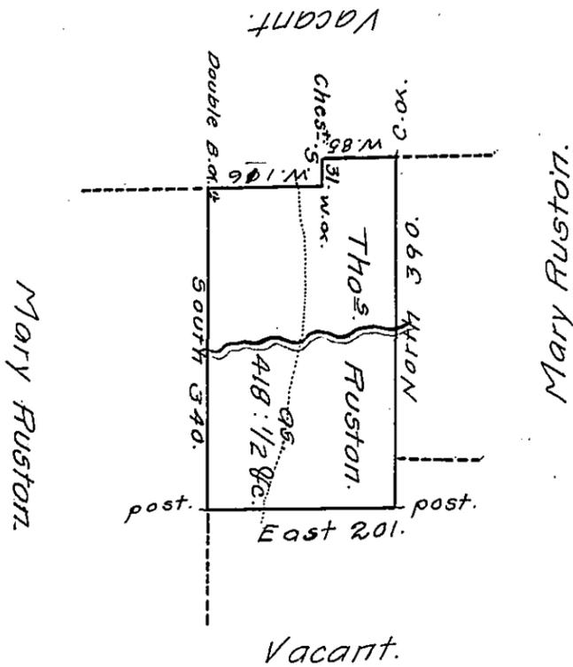
A draft of a tract of land called \_\_\_\_\_ situate on the South Branch of Roring Creek in Northumb<sup>d</sup> County Containing Four Hundred & Eighteen acres 1/2. Surveyed for Thomas Ruston the 3<sup>rd</sup>. day of October, 1793 by virtue of a Warrent dated the 11<sup>th</sup>. day of June, 1793.
